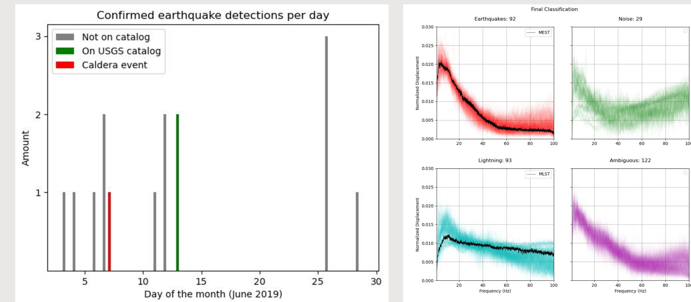
Figure 8: Cross-referencing the analysis from figure 6, events were appropriately classified. Results are confident that 92 of the events are earthquakes and should be further studied. Another 122 events are still unclassified and can be evaluated using more complex methods, if necessary.
