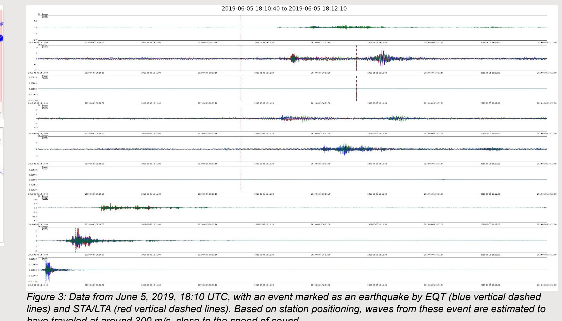
Figure 3: Data from June 5, 2019, 18:10 UTC, with an event marked as an earthquake by EQT (blue vertical dashed lines) and STA/LTA (red vertical dashed lines). Based on station positioning, waves from these event are estimated to have traveled at around 300 m/s, close to the speed of sound.
