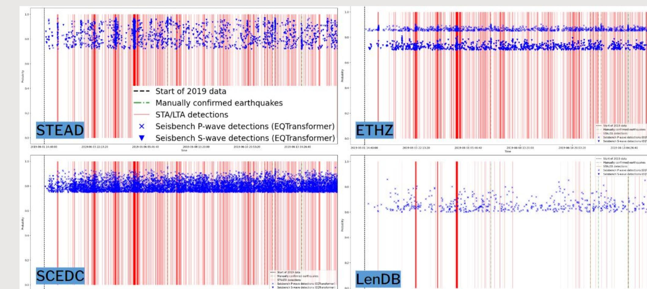
Figure 2: Comparison of returned picks from the four different EQTransformer models tested.
