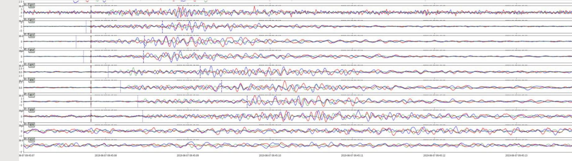
Figure 5: Waveform of a possible local earthquake. Wave arrivals suggest very high hypocentral proximity.
