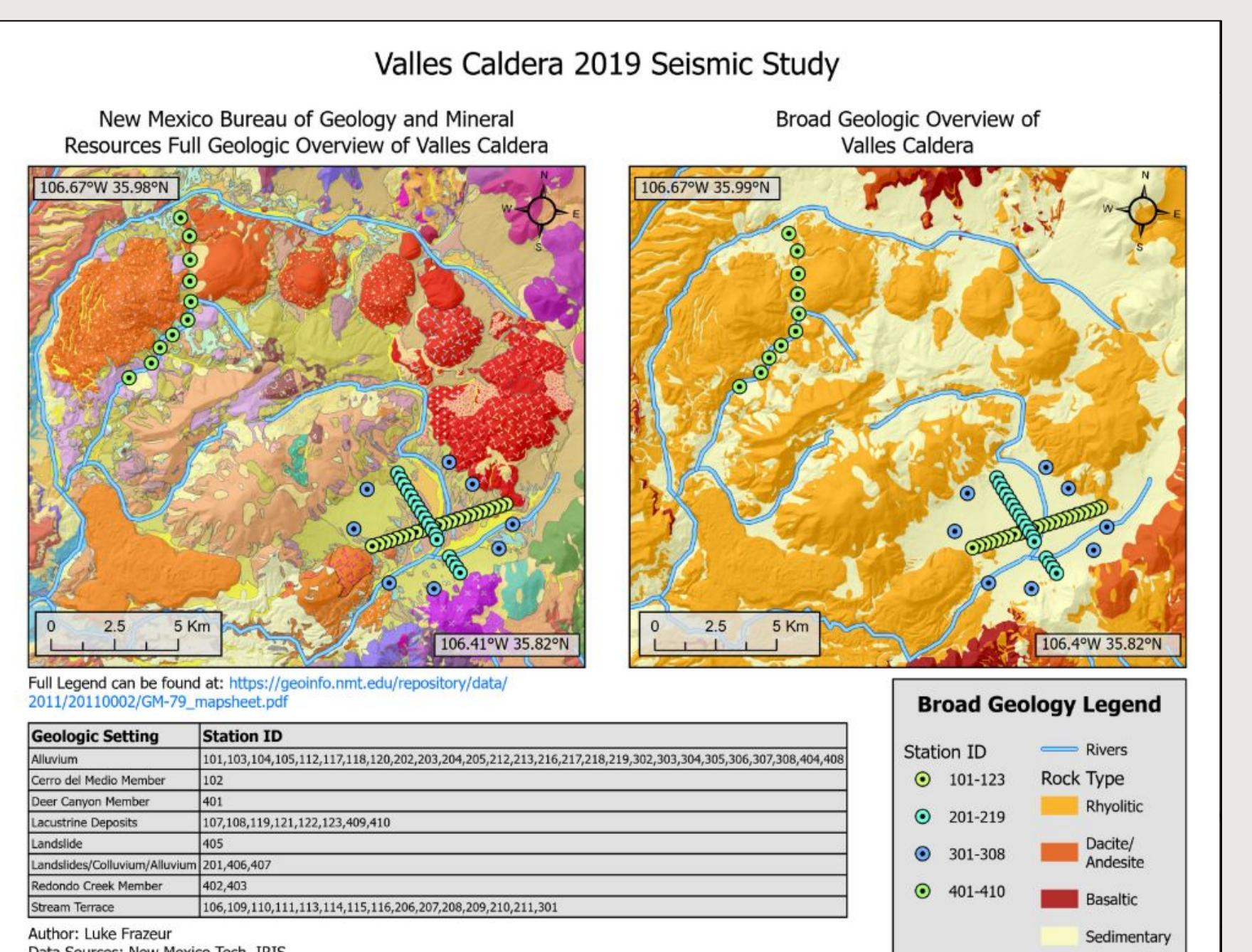
Figure 1: Map figure depicting geophone locations and geology of the region. The map on the left shows the detailed geologic map developed by the NM Bureau of Geology and Mineral Resources. The map on the right is a simplified derivation developed by the author. Geophones are mostly set in sedimentary rock which can account for slightly slower wave speeds, however the subsurface is still mostly igneous. Stations 401-410 are separated from the others by over 10 kilometers.
